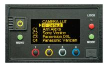
Since digital cameras use different sensors in their image capture, there are differences between cameras on how they capture LED lighting. The **Camera LUT** is a way of harmonizing the Kino Flo LED light sources to the camera. Depending on the camera and the Kelvin setting, some differences are very subtle, while others can be more dramatic.
