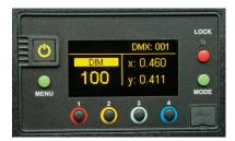
The **CIE xy** mode determines the color displayed by its CIE xy coordinates. This mode is a means to adjust Kino Flo LED products to other manufacturers' lighting products that also have a CIE xy function or by using a color meter for comparison.
