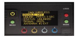
The LED Controller/Fixtures include a built-in Lumen Radio receiver and can be operated wirelessly with a Lumen Radio transmitter (sold separately). For more information on Lumen Radio Receiver/Transmitter, see www.LumenRadio.com.
