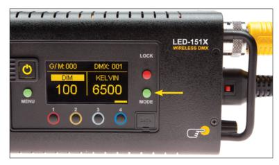
Press the Mode button to select **Dim**. Rotating the control knob will dim the light of the fixture. Default setting is Fine. Press the Control knob to toggle between **Fine** and **Coarse** increments or when selecting options within menus. When the power is turned off or removed, the display will remember its last setting.
