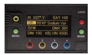
In  ${\bf Gels/Hue}$  mode (in addition to  ${\bf G/M}$  control),  ${\bf Gel},$   ${\bf Hue}$  angle and  ${\bf Saturation}$  adjustments are available.
