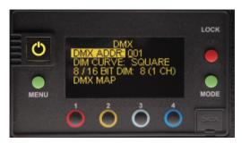
Press the Menu button to select **DMX**. Press and turn the control knob to select individual digit settings for a valid address from 1-512. On the main display, "**X**" next to DMX indicates DMX signal is present.
