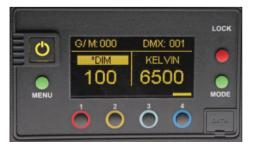
The default setting for **DIM** is that smoothing is on. When smoothing is on, it introduces a time lag such that the individual dimming steps are less noticeable. However, when working in DMX and instant response is required, it is recommended that smoothing be turned off.
