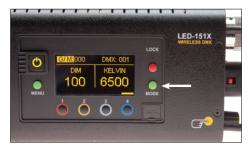
Press the Mode button until **G/M** is highlighted. Rotating the control knob to the right will adjust towards Green. Rotating to the left will adjust towards Magenta. Default setting is Fine. Press the Control knob to toggle the G/M from **Fine** to **Coarse** increments.
