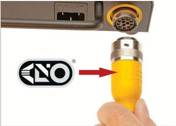
The harness connects directly to the controller. Connect the harness to the controller. Align the key ways on the harness connector with the oval **Logo** at the top with the circular receptacle on the ballast. Rotate the silver locking ring until it clicks into the lock position.
