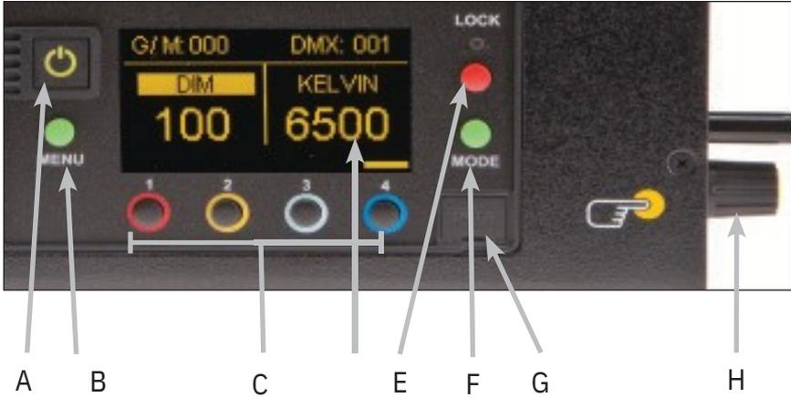
**A) On /Off:** **On** = Green light displayed. **Off** = Red light displayed. The display and all menu settings can be operated while the power button is in the Off position, as long as power is applied to the controller. The On /Off button only controls the light source.
