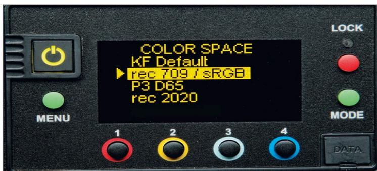
**Color Space** defines the RGB color space used and only affects color – not Kelvin. It is used in **RGB** mode and **Hue Angle** and **Saturation**. The RGB color space defines the value of Red, Green, and Blue primaries (in CIE xy) and the white point is fixed at 6500 Kelvin.
