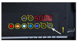
Press the **On/Off** button to turn on the fixture. The display will show its last setting.
