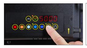
To reset factory settings, press and hold the **LOCK** / **RESET** button for 5 seconds.
