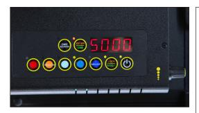
The Celeb 401Q DMX operates on two DMX channels using DMX512. The first channel operates dimming; the 2nd channel operates Kelvin color temperature control.
