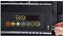
Turn the dimming knob to select a valid address from 1-512. (Note: 0 or 513-999 are invalid addresses.)
