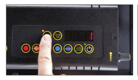
To save the DMX channel, press the **DMX ADDRESS** button again. When set, the displayed number will stop flashing.
