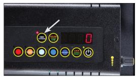
Press and hold the **DMX ADDRESS** button to select a
