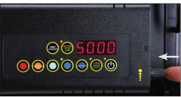
Press the rotating knob once to shift the **Kelvin** profile from **Coarse** to **Fine** increments.
