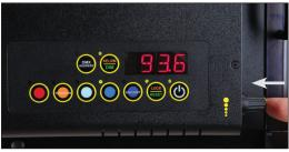
Press the rotating knob once to shift the **Dim** profile from **Coarse** to **Fine** increments.
