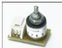
6110044 VistaBeam 610 Lamp Selector SW
