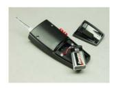
Pull down lock tab. Remove the back panel and insert a 9-volt battery (included).
