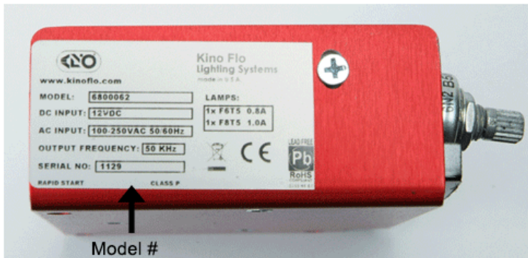
Mini-Flo 239X Ballast Board (Part # 6800062) Side View
