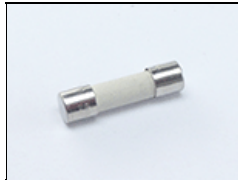
1300030 Fuse 5x20 Cer Slowblow 10A/250V for 1270383 (2 required)
