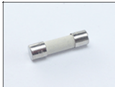
1300022 Fuse 5x20 Cer Slowblow 6.3A/250V for 1270383 (2 required)
