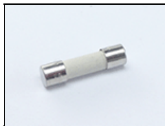
1300022 Fuse 5x20 Cer Slowblow 6.3A/250V for 1270383 (2 required)
