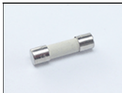
1300022 Fuse 5x20 Cer Slowblow 6.3A/250V for 1270383 (2 required)
