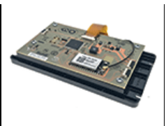
6800251 LED Controller w/ Timo Antenna
