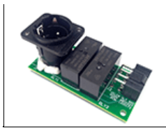
6800224 Celeb Relay Control Board. Used in Rev B or higher. (Replace w/ same)
