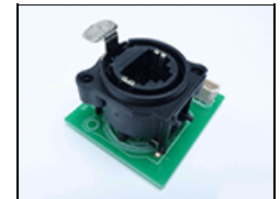
4010020 Celeb Remote Board (NE8FAV). Used in Rev A & B. (Replace w/ same.)
