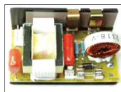
6800042 12VDC BAL-140 Ballast
