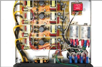
5) Install new ballast board, three (3) nuts,
