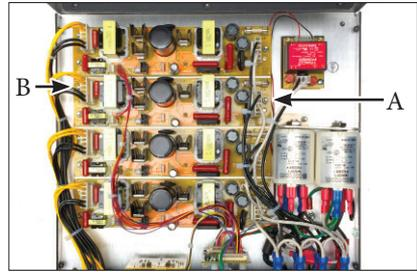
2) Remove AC input connector (A).
