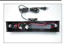
4) Install new ballast board. (Note: Do not remove protective cardboard.)
