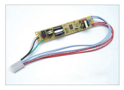
The **DS1** Ballast Board is to be used as a replacement ballast board for the Desk-Lite model # **DES-121**. Use part # **6800190** for 120VAC and part # **6800191** for 230VAC. For latest warranty information, see the Kino Flo website at **www.kinoflo.com**
