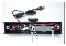
2) Remove three (3) ballast board screws.
