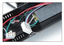
3) Remove AC input/output connector and remove old ballast board.
