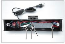
5) Install AC input/output connector and three (3) ballast screws.
