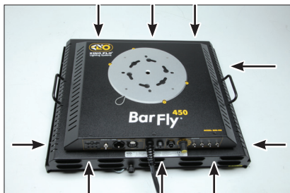
1) Remove ten (10) cover screws.
