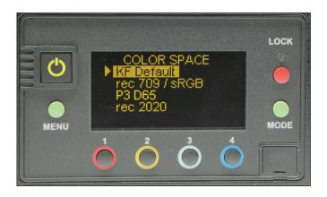
**Color Space** defines the RGB color space used and only affects color – not Kelvin. It is used in **RGB** mode and **Hue Angle** and **Saturation**. There are a few instances in the FX (Effects) mode that are also affected when color is used. The RGB color space defines the value of Red, Green, and Blue primaries (in CIE xy) and the white point is fixed at 6500 Kelvin.
