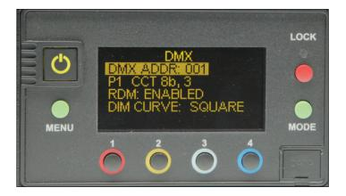
Press the Menu button to select **DMX**. Press and turn the control knob to select individual digit settings for a valid address from 1-512.
