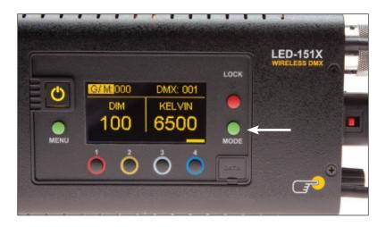
Press the Mode button until **G/M** is highlighted. Rotating the control knob to the right will adjust towards Green. Rotating to the left will adjust towards Magenta. Default setting is Fine. Press the Control knob to toggle the G/M from **Fine** to **Coarse** increments.
