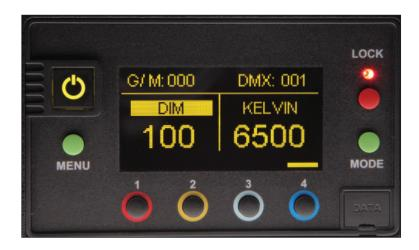
Press the **Lock** button to lock the Dim, Kelvin and G/M setting (Applies to White, Gels/Hue, RGB, FX or CIE xy Modes). A red indicator light will display in Lock mode. Manual controls will be disabled. To unlock, press the Lock button again. The red indicator will turn off.
