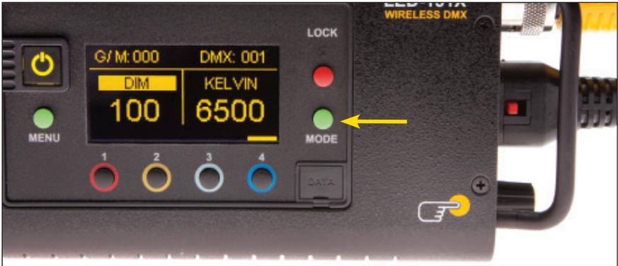
Press the Mode button to select **Dim**. Rotating the control knob will dim the light of the fixture. Default setting is Fine. Press the Control knob to toggle between **Fine** and **Coarse** increments or when selecting options within menus. When the power is turned off or removed, the display will remember its last setting.
