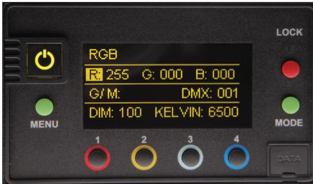
In **RGB Color** mode (in addition to G/M control), individual RGB (Red, Green, Blue) adjustments are available. Press Menu, select General and press control knob to change Mode to RGB.
