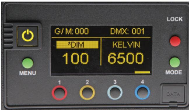
The default setting for **DIM** is that smoothing is on. When smoothing is on, it introduces a time lag such that the individual dimming steps are less noticeable. However, when working in DMX and instant response is required, it is recommended that smoothing be turned off. The **\*DIM** designates that the smoothing function is off.
