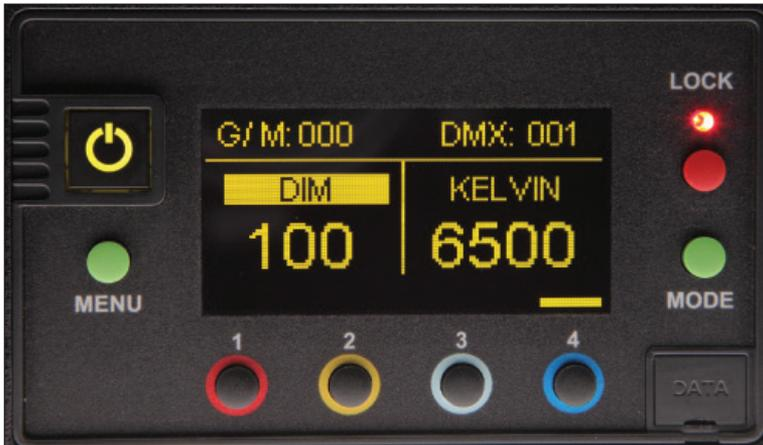
Press the **Lock** button to lock the Dim, Kelvin and G/M setting (Applies to White, Gels/Hue, RGB, FX or CIE xy Modes). A red indicator light will display in Lock mode. Manual controls will be disabled. To unlock, press the Lock button again. The red indicator will turn off.
