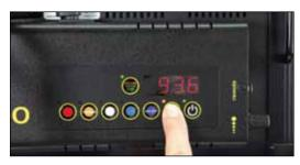
Press the LOCK / RESET button to lock the Kelvin and Dim settings. An amber indicator will display in LOCK mode.
