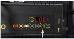
In **LOCK** mode, controls are disabled and **LOCK** will appear in the display.
