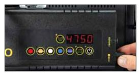
In **KELVIN** mode, the Kelvin can be fine tuned with the adjustment knob to any custom settings between 2700 to 5500.
