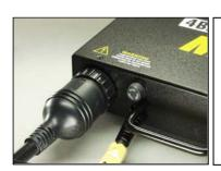
To insert the cable **(X19-25M)**, align the key ways on the extension cable with the circular receptacle on the ballast. Rotate the locking ring until it clicks into the lock position.
