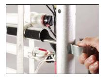
To give rigidity to the Blanket-Lite insert 4 pins through the pipe frame into the two horizontal Blanket-Lite harness tubes.
