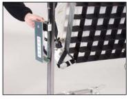
Using the Mafer Clamp (MTP-AME58) mount the Hanger onto the stand.
