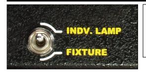
Setting the Ballasts to "Fixture Mode" allows the user to turn lamps on and off with an "inside-out" pattern from a dimmer board.
