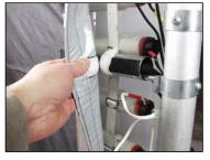
Orient the reflector so that the Velcro strips on the reflector line up with the Velcro on the Lamp harness tubes.
