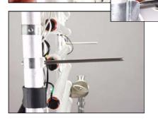
Insert the remaining 8 pins at 90 degrees to the frame. These pins support additional accessories.
