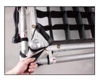
Set the tension of the louver by adjusting the four Velcro loops.
