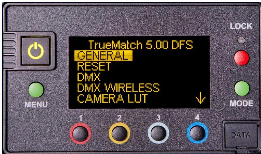
*Photo: Controller display showing True Match 5.0 with RDM capability.*
