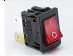
1290055 Switch Rocker Mini DPST 12A 250V. Used in Rev C or higher. Replace w/ same.
