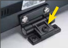
Fixture hinge tension is adjusted by the central Phillips head screw.
