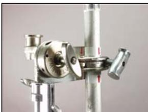
Clamp the two frame ears between the two arrows found midway on the pipe frame. Face in the same direction as the frame corners.
