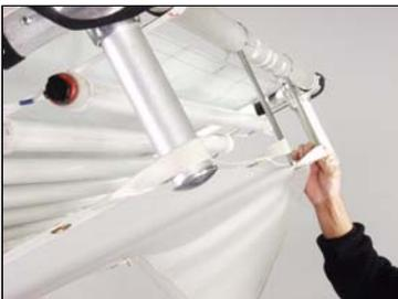
The pins along the middle of the frame provide additional support to the diffusion.
