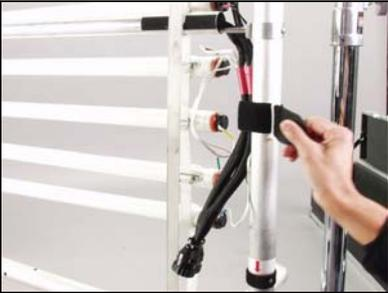
Use the Harness Velcro straps to secure the harnesses to the frame.
