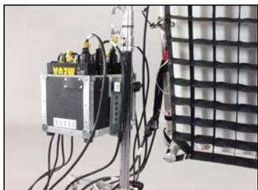
Connect the extension cables to the harnesses and ballasts. (See Page 9)
