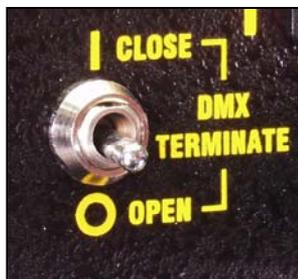
The **DMX Terminate Switch** must be set to open ( **O** ) on Ballasts within the DMX chain.
