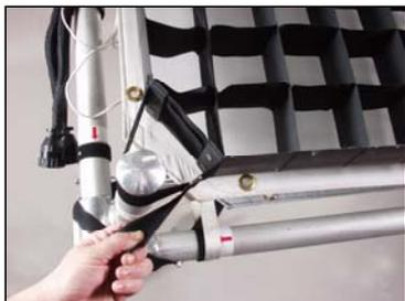
Set the tension of the louver by adjusting the four Velcro loops.
