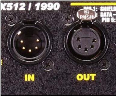
Any theatrical lighting board with DMX 512 protocol can be used to individually turn **on/off** lamps in a Fixture.
