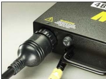
To insert the cable (**X19-25M**), align the key ways on the extension cable with the circular receptacle on the ballast. Rotate the locking ring until it clicks into the lock position.
