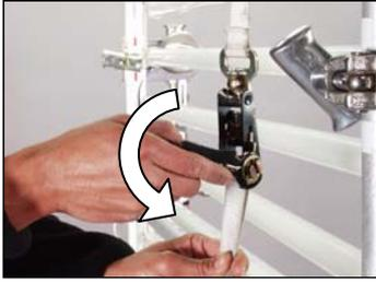
6) Draw up any slack in the strap and tighten by drawing down the ratchet lever until tight.
