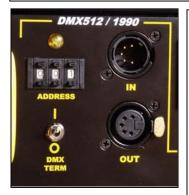
Any theatrical lighting board with DMX 512 protocol can be used to individually turn **on/off** 12 lamps per Multi-Flo.
