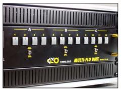
12 manual switches control individual lamps that are grouped into three 4-Lamp circuits (A, B, C).
