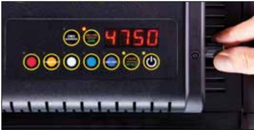
In **KELVIN** mode, the Kelvin can be fine tuned with the adjustment knob to custom settings between 2700K to 5500K.
