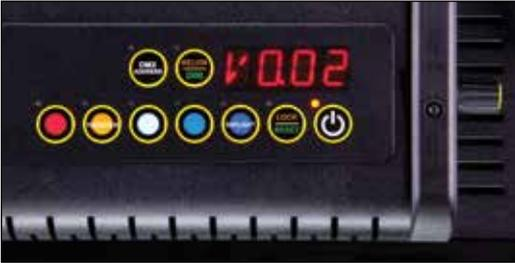
When power is first applied to the fixture, the alphanumeric display shows the current software version.
