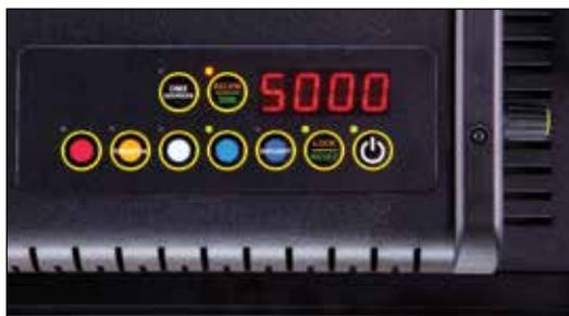
The Celeb 400Q DMX operates on two DMX channels using DMX512. The first channel operates dimming; the 2nd channel operates Kelvin color temperature control.
