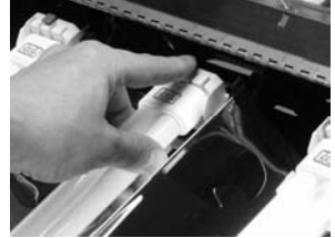
To release lamps, press Red button and lift lamp out.
